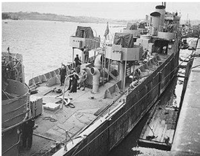
HMS Campbeltown being converted for the raid. There were twin lines of armour plate down each side of the ship to protect the Commandos. Two of her funnels have been removed, with the remaining two cut at an angle.
